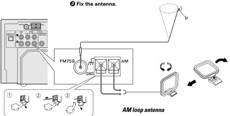
The supplied antenna is for indoor use. Place it as far as possible from the main system, TV set, speaker cords and power cord, and set it to a direction which provides the best reception.
